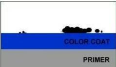
Surface contamination, as shown by this diagram, is difficult to clean or polish off, yet a detailing clay bar can remove it with ease.
